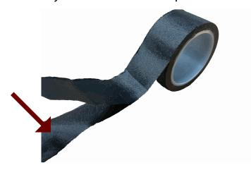
3. Apply adhesive side of fusion tape to cable surface. Wrap tape in a spiral, stetching enough to create a tension that conforms to the cables. Overlap each turn roughly 50% until the connection is completely encased in tape.
