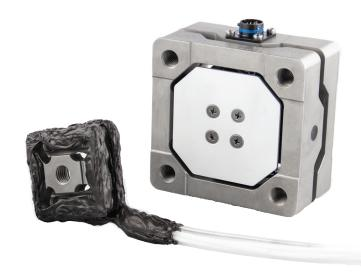
Each load cell transducer is machined from a solid block of stainless steel or aluminum, which ensures excellent linearity throughout the entire force range, as well as minimal hysteresis. Weatherproof coatings are applied to all strain-gauged surfaces to ensure the load cell will survive in almost any environmental condition experienced in industrial or automotive applications.
